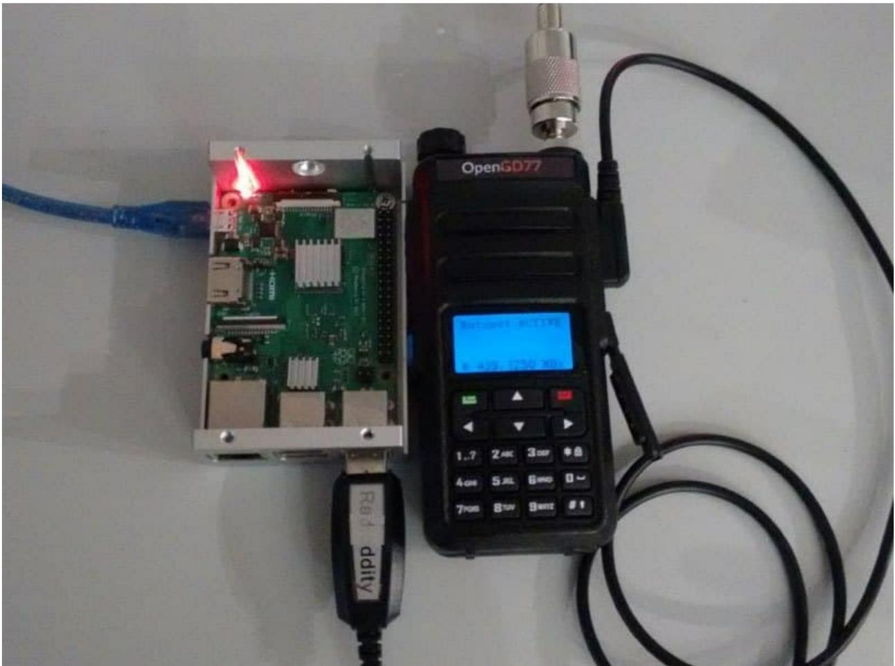
Hotspot mode works with the Raspberry Pi Zero, but a adaptor cable is needed to convert from the micro USB port on the RPi Zero to the full size USB plug on the radio's programming cable.
