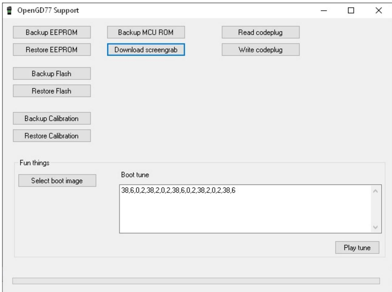
From here you can backup, the internal 64k EEPROM and the 1 mega byte Flash chip, as well as Reading and Writing the codeplug. The calibration data store in the Flash chip (At address 0x8f000) can be backed up and restored without backing up the whole of the Flash.
