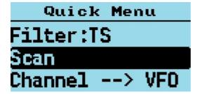
Pressing the **Orange** button on the top of the radio in VFO mode displays the Quick menu for the VFO screen. Currently this has five options.
