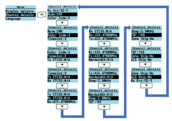
Pressing the GREEN key enters the menu system, press again to enter a menu subsection or to exit the menu.
