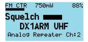
Once in squelch control mode, pressing **Right** tightens the squelch incrementally, **Left** opens up the squelch incrementally. The VFO and each channel have individual squelch settings that can be set in this manner.
