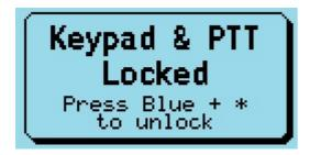
You can also lock the PTT button by pressing the **Green** menu key to display the Main menu and then pressing the **Hash (#)** key. The keypad and the PTT can both be locked at the same time by first locking the PTT and then the keypad.
