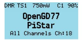
Pressing the  ${\bf Up}$  and  ${\bf Dow}\,{\bf n}$  arrows will cycle though all channels in the zone.
