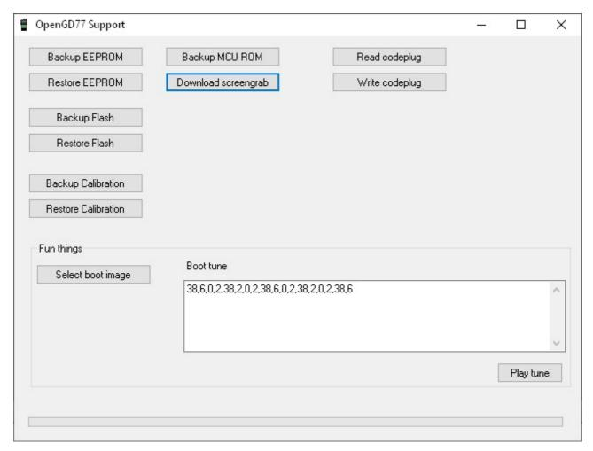
From here you can backup, the internal 64k EEPOM and the 1 mega byte Flash chip, as well as Reading and Writing the codeplug. The calibration data store in the Flash chip (At address 0x8f000) can be backed up and restored without backing up the whole of the Flash.
