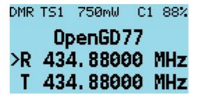
The frequency used in the VFO for both Tx and Rx will be read from the "VFO A" settings of the codeplug.
