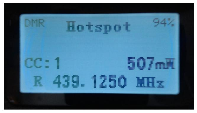
If the radio does not enter Hotspot mode, power cycle the radio and power cycle PiStar
